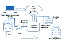
Figure 1. Flow chart of a PEF food processing system with basic component (Maged *et al.*, 2012)
